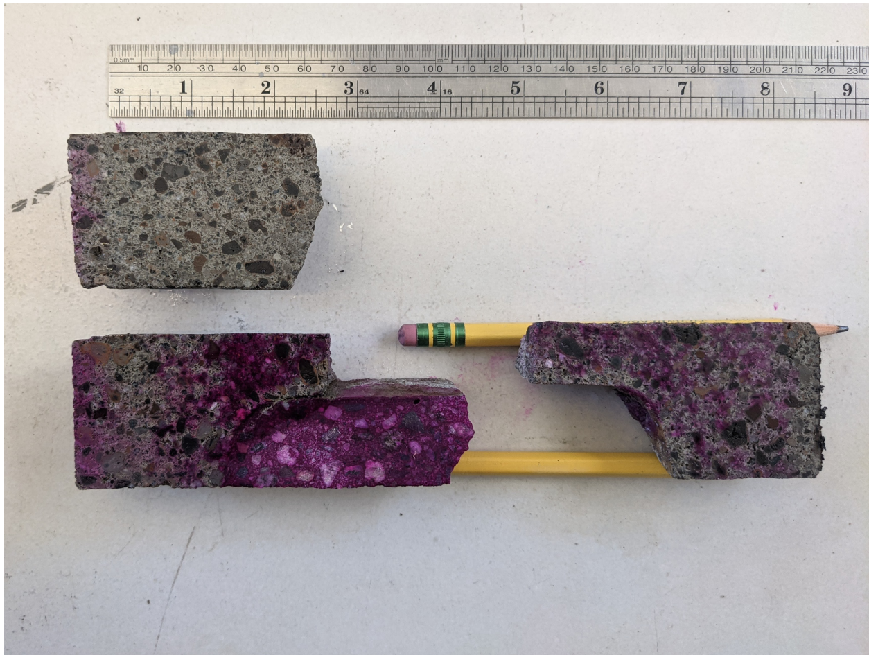
Figure 3. Comparison of freshly cut cross sections of the reference (top, B2) and the OXO H2O treated (bottom, A3) cores. The color change of the phenolphthalein indicator to pink is clearly visible throughout the treated CMU core (A3).
